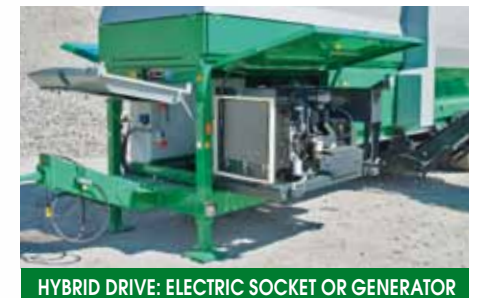
HYBRID DRIVE: ELECTRIC SOCKET OR GENERATOR
